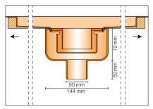
Longitudinal view of wall/intermediate installation
